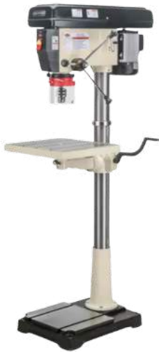
SHOP FOX M1039 20" DRILL PRESS 1.5 HP 110/220 12 SPEED 180-3240 RPM
