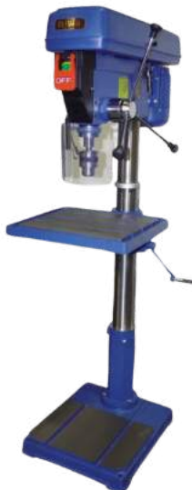
SHOP FOX M1039 20" DRILL PRESS 1.5 HP 110/220 12 SPEED 180-3240 RPM
